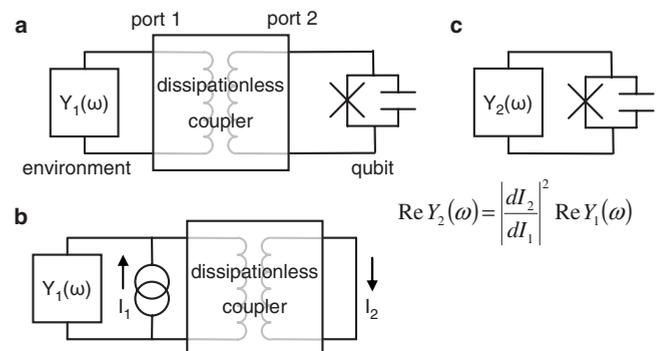
FIG. 1. Impedance transformation by a two-port dissipationless coupler. (a) Qubit is connected through a dissipationless coupler to environment, described by admittance  $Y_1(\omega)$  of the external circuitry. (b) The transfer function of the coupler relates current source  $I_1$  across the input port to current  $I_2$  across the shorted output. (c) The effective dissipation seen by the qubit at port 2 is transformed by the squared derivative of the transfer function.
