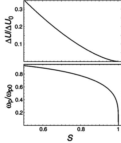
FIG. 2. Barrier height and plasma frequency as a function of the dimensionless bias current  $s$ . Here  $\Delta U_0 \equiv 2E_J$  is the barrier height at zero bias, and  $\omega_{p0}$  is the zero-bias plasma frequency defined in Eq. (12).
