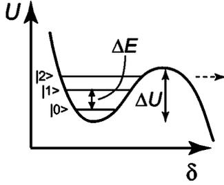
FIG. 3. Metastable potential well in the cubic limit, showing the barrier of height  $\Delta U$  that separates the metastable states  $|0\rangle$ ,  $|1\rangle$ , and  $|2\rangle$ , from the continuum. This figure applies to the case of bias currents  $s$  just below 1. The lowest two states are separated in energy by  $\Delta E$ .
