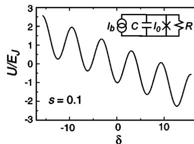
FIG. 1. Effective potential  $U(\delta)$  for dimensionless bias current  $s \equiv I_b/I_0$  equal to 0.1, plotted in units of  $E_J$ . Inset: Equivalent-circuit model for a current-biased Josephson junction. A capacitance  $C$  and resistance  $R$  are in parallel with an “ideal” Josephson element, represented by a cross and having critical current  $I_0$ . A bias current  $I_b$  is driven through the circuit.
